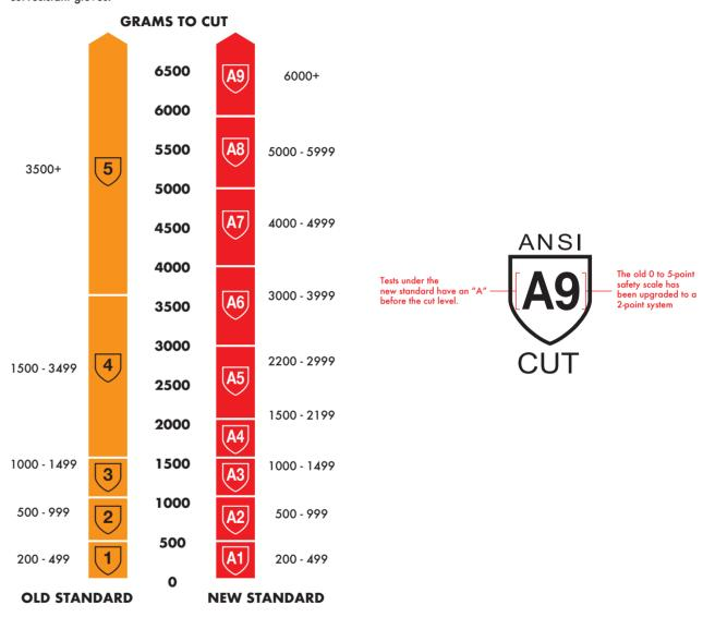
The old standard measured the weight in grams for a blade to cut material with either a Cut Protection Performance Tester (CPPT) or a Tomodynamometer Test Machine(TDM). The new standard allows only one type of machine, TDM-100, to be used.
